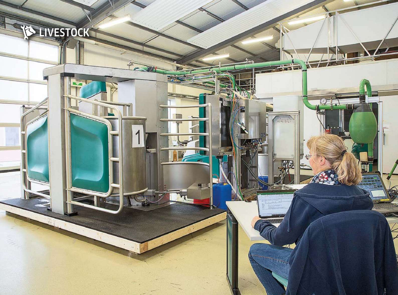
Gea's latest single-box milking robot, the Monobox DairyRobot R9500 Edition 2021, was put through the DLG test last September.
