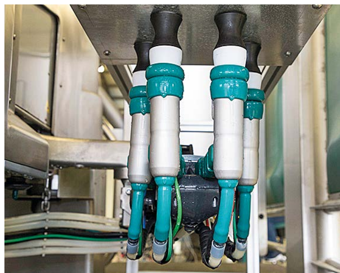
No brushes required here – the Gea system cleans the teats inside the cups.
