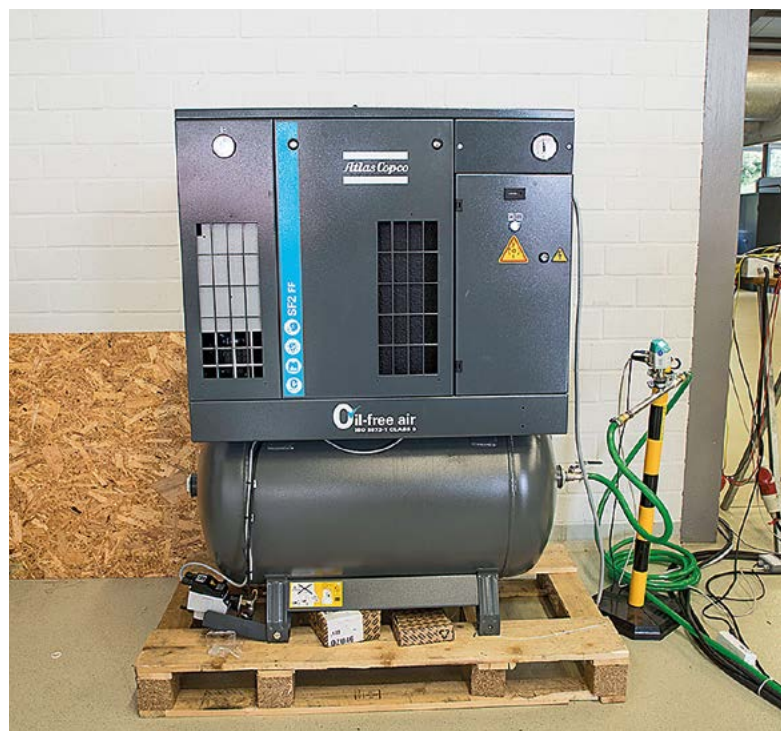
The Atlas Copco SF22 compressor has a nominal output of 2.2kW.
