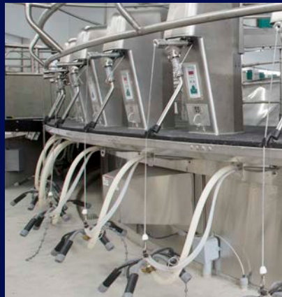
PosiForm Drop-down Hose Support — drops units below the deck when not milking and out of the way of the operator.
