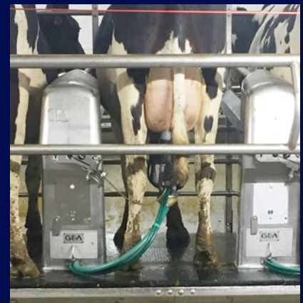
PosiGuide Non-drop-down Hose Support — milking units stay above the deck after removal from the cow.
